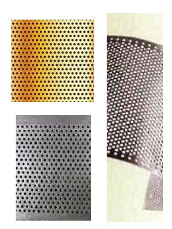
Perforated metal, also known as perforated sheet, perforated plate, or perforated screen, is sheet metal that has been manually or mechanically stamped or punched to create a pattern of holes, slots, or decorative shapes. Materials used to manufacture perforated metal sheets include stainless steel, cold rolled steel, galvanized steel, brass, aluminum, tinplate, copper, and more.
